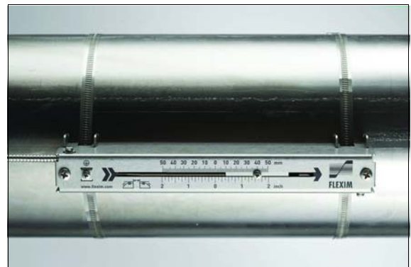
Measurement with transducers mounted by PermaRail
