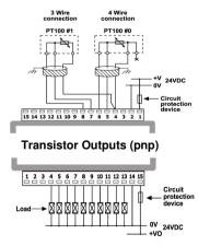
The 0V signal of the analog input and output must be connected to the controller's 0V.
