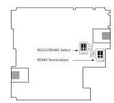
Note: it is possible to establish a PC to PLC connection using RS232 even when the PLC is set to RS485 (it will eliminate the need to open the controller for jumper setting). To do so, removes the RS485 connector (pins 1 & 6) from the PLC and connect a standard RS232 programming cable instead. Note that this is possible only if DTR and DSR signals of RS232 are not used (standard case).
