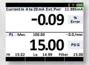
mA loop span. For example, if you are testing a 30 psi full scale pressure transmitter with a corresponding 4-20 mA signal, you can program into the calibrator a 0 to 30
