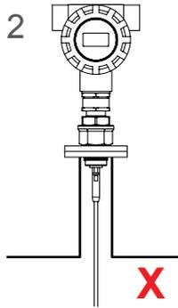
1. Stand pipes protruding into vessel may cause signal interference. Digitisation and / or Blanking Distance must be adjusted to avoid measurement issues
