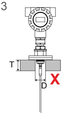
3. Roof Thickness (T) should not exceed Diameter (D) of cut away. Digitisation and / or Blanking Distance must be adjusted to avoid measurement issues
