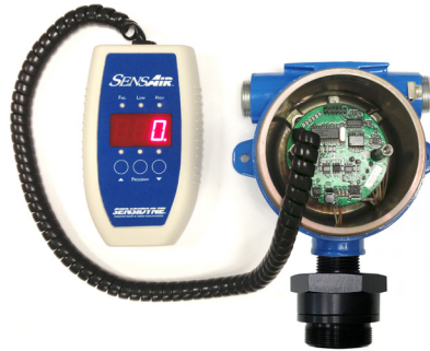
Hand-held Controller (821-0701-01-R) provides local interface for blind (non-display) models.
